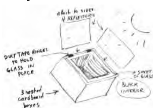
A solar oven design made with cardboard boxes, aluminum foil, and a piece of window glass. Interior of the box is flat black paint.
